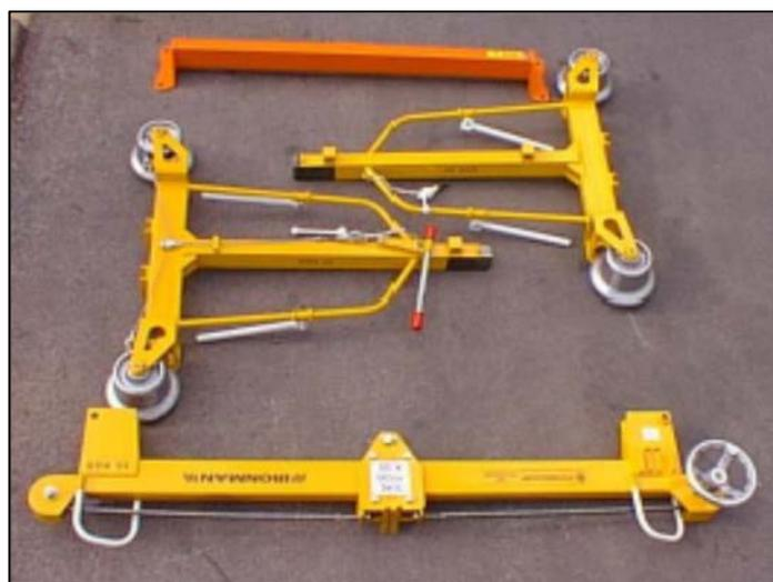
Figure 2: Ironman broken down into its four main parts
